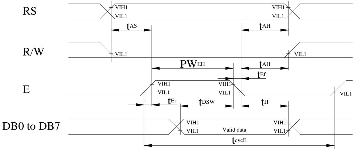
$T_a=25^{\circ}\text{C}, V_{dd}=5.0\pm 0.5\text{V}$
